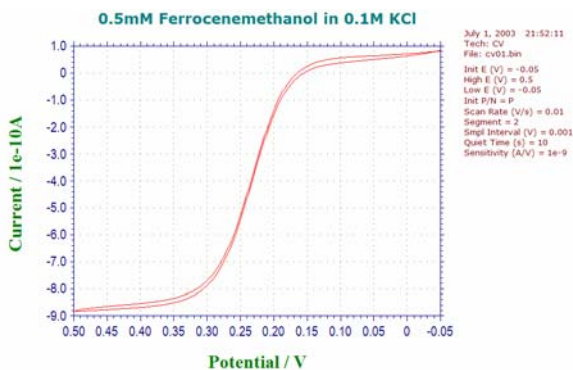
Cyclic voltammogram at an ultramicroelectrode.
